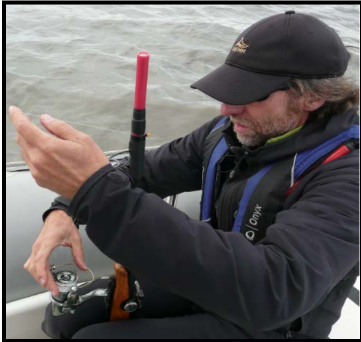
Figure 10. The plastic cylinder and dart assembly was tethered with a fishing line spooled on a fishing reel attached to the forestock of the rifle. The reel was used to retrieve the plastic cylinder and dart containing the biopsy sample (photo: LGL).
